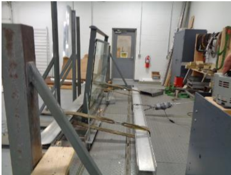
Photo No. 4 In-Fill Load Test at Bottom of Glass In-fill
