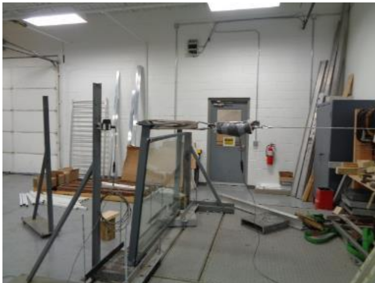
Photo No. 2 Concentrated Load at End of Top Rail (Rail to Post Connection/Post)
