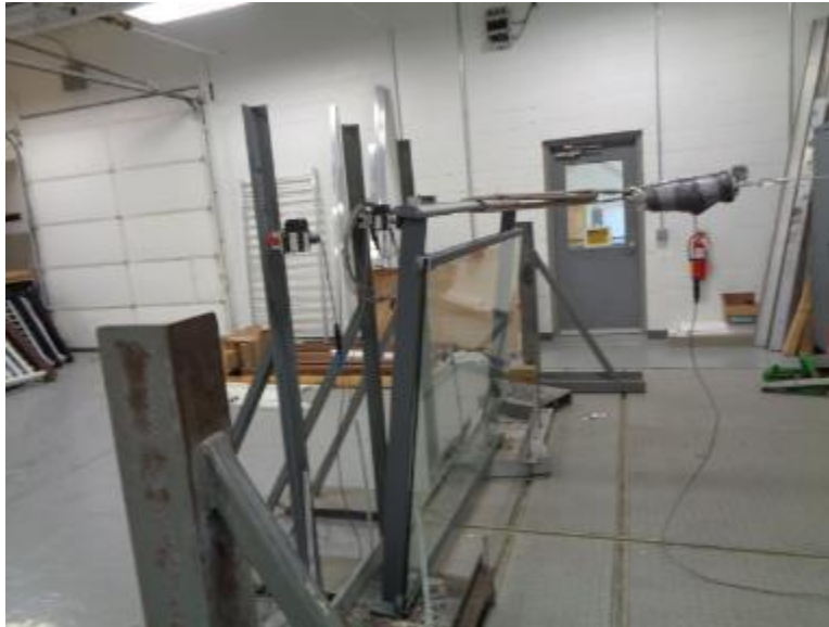
Photo No. 1 Concentrated Load Test at Mid-Span of Top Rail
