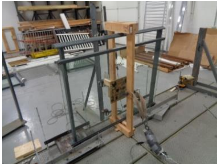
Photo No. 3 In-Fill Load Test at Center of Glass In-fill
